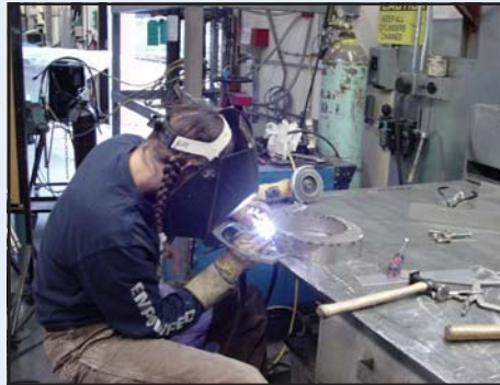
Tamara Carter welds stainless steel lettering.
